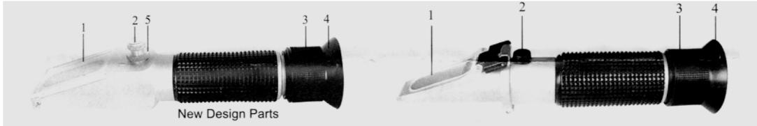
1----Daylight Plate; 2----Calibration Screw; 3----Focus Adjustment; 4----Eyepiece; 5----Calibration Screw Block
