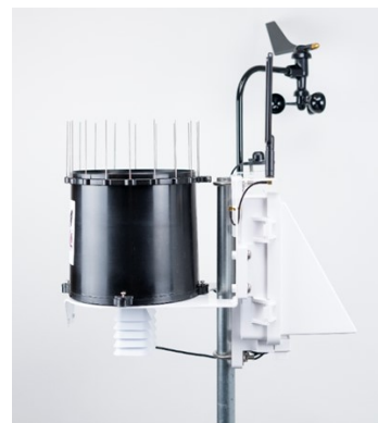
ET Station. The Weather Station and Rain Station have the same design with different sensor sets.
