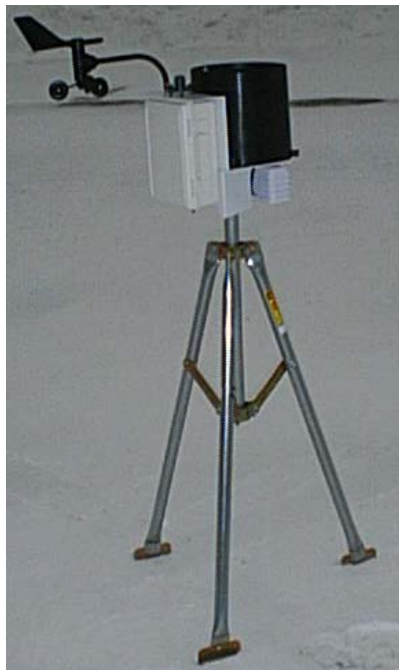
Weather Station mounted on tripod
