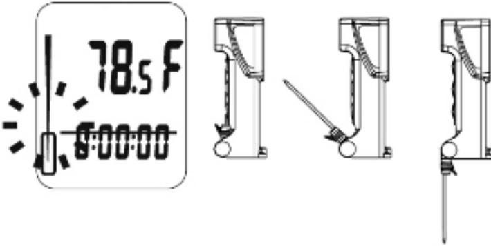
and insert into the target at least 1/2" (10mm) deep for several seconds or stir the liquid to equilibrate with the target object, and then press MEAS to measure internal temp. The probe icon blinks while measuring and stops with short beeps when the readings stabilize.
